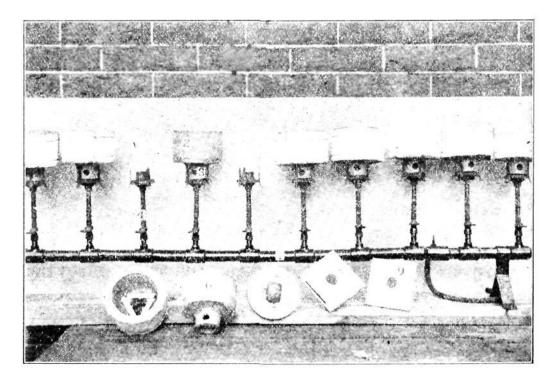
the bottom, its object being cleanliness. But less-costly graphite covers answer quite as well. In the center of each lid is a vent-hole of about 3 cm. diameter. The muffles may be of any size. Ours have the following dimensions: The main body or re-
